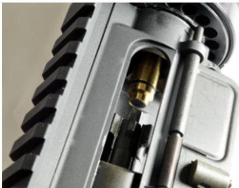
The LT-223 fits inside the cartridge chamber and features a firing-pin activated switch that indicates bullet impact with a bright red laser dot. A built-in snap cap protects the firing pin and O-rings hold the laser accurately in place allowing for repeated dry fire practice without compromising accuracy. The rim-less cartridge trainer also allows for constant racking without unintentional ejection.
